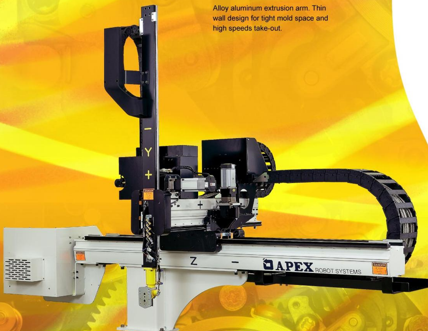
All moving axis rides on harden tool steel rail with bearing guide. Less friction quiet smooth movement ideal for high speeds application.
